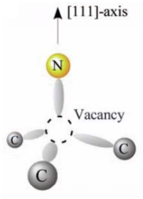
Three qubits: NV + ^{13}\text{C} + ^{13}\text{C}
